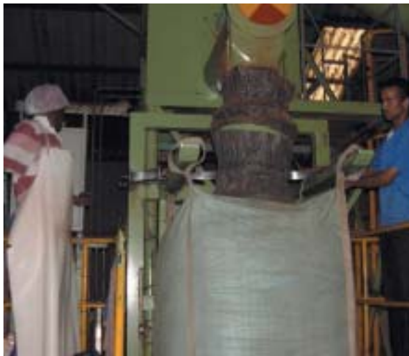
Fig. 1. Bulk loading and bagging of fishmeal causes spillage and aerosolised dust particulate if inadequately removed by local exhaust ventilation systems, resulting in work-related asthma.
